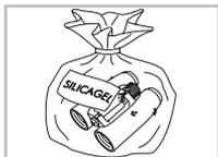
If the instrument is wet, it must be dried prior to storage.
