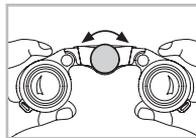
It is possible to bring every subject into focus from the shortest adjustment distance (see Technical Data Sheet) to infinity by turning the focusing wheel.
